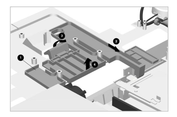
Figure 6-34. Removing the Puller Plate Assembly
